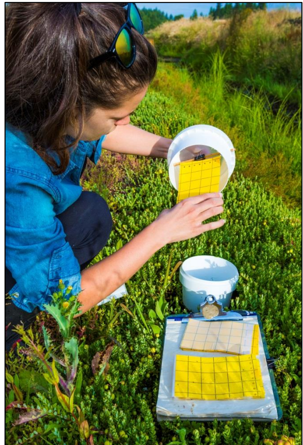
Figure 1. (Clockwise from top left). Exploded view of cylindrical emergence trap , showing top bucket and suspended yellow sticky card that slide into bottom bucket with its dark ground cloth skirting and wire pegs. The yellow sticky card is covered in protective paper that is removed as the trap is installed in the field. View of trap anchored into cranberry field , showing top bucket with mesh lid sliding into bottom bucket. The end of the dowel is visible on the lip of the lid of the top bucket. The foldback clip on the dowel can be seen through the mesh on the lid. Miranda Elsby removing double-sided yellow sticky card from top bucket and preparing to install a new yellow sticky card.
