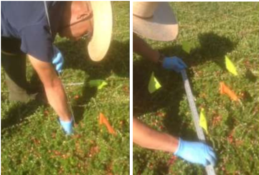
Figure 6 (left): Conducting pull-test to measure the height of the canopy lifted. Figure 7 (right): Measuring the area of the canopy lifted by the test.
