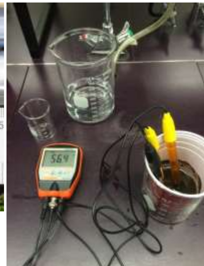
Figure 2(right): Soil chemistry meter and sensor measuring pH and Redox potential of a sample.
