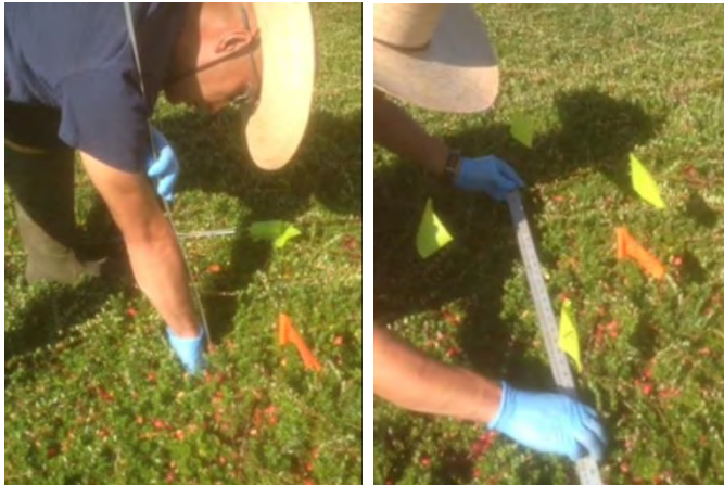
Figure 2-3 (left): Conducting pull-test to measure the height of the canopy lifted.
